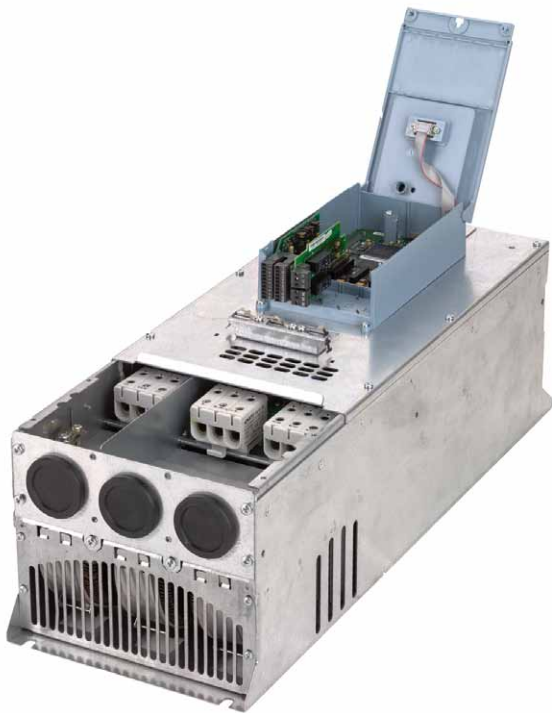
Drives application including our Ensto Clampo Pro three-pole terminal blocks specially designed to meet the needs of the drives industry.
